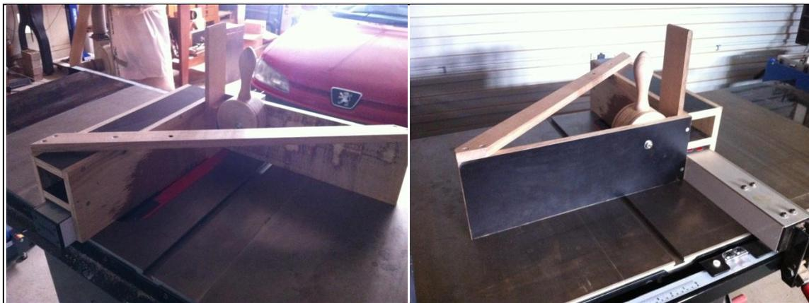
The tenoning jig to cut the joinery for the drawers.
