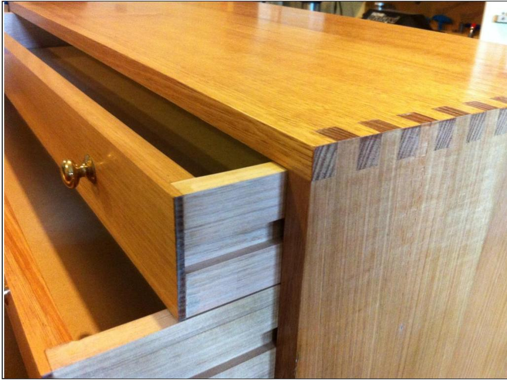
Detail of the joints used for the carcass of the drawers
