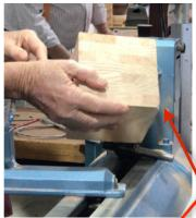
This project requires a cube as the blank. To get a blank large enough (rather than sacrificing a large log) Ron created one by laminating finished pine & meranti boards.
