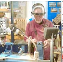
The rubber coated plate provides the friction to turn the piece while a vacuum cleaner or similar suction device holds it to the lathe. To help centre (& hold) the piece as with the second method the tailstock & a live centre or a chuck on a threaded live centre can be used.
