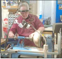
For this method to work the rim needs to be trued up and smooth to allow the suction device to be effective.
