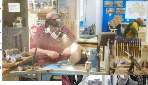
1. After working the inside of the bowl to true that up a shelf / channel can be cut that allows the bowl to be held using:
