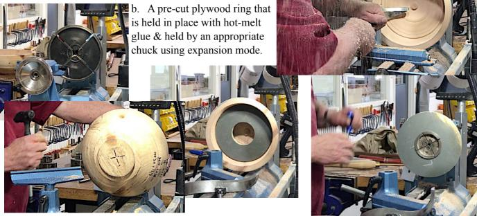
2. The next mounting method is to use a shaped piece of plywood attached by faceplate or using a turned foot to mount with a chuck.
