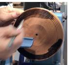
Ron started out simply by using a reverse ground 6mm bowl gouge 'beading tool' to put a series of beads into his test piece. He then used ebonizing fluid and sand paper to give a dark ring affect. Then, so he could do something different, he just turned the texturing off to have a blank slate.
