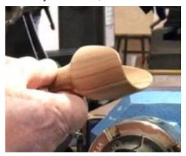
Mount your timber on the lathe and cut a tenon on the end to fit your scroll chuck. Put in the chuck and turn to a cylinder (using the tailstock for safety).
