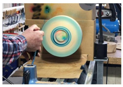
He then cleaned the airbrush with water, leaving the piece spinning to give it time to dry. The next colour is then applied.
