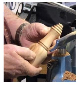
Now work out which part of the scoop will be removed. This was done using a sanding disk on the lathe with coarse paper. (Obviously, this could also be done with a stationary belt sander.)
